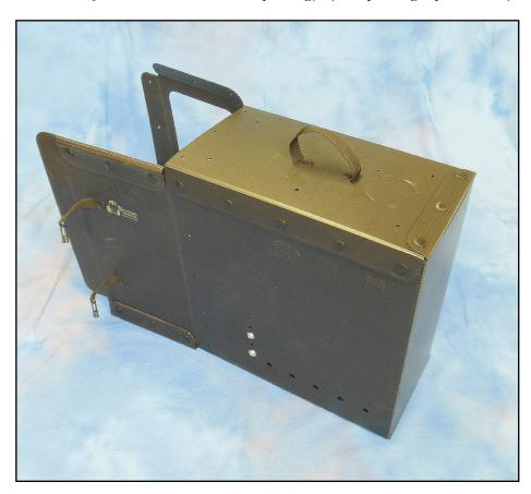
7. Next, join the Back panel to the Top and Bottom panel by folding over the flaps and riveting together. (See photograph above.)
