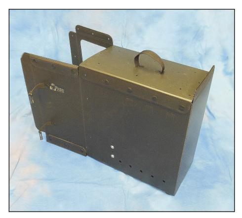
6. Next, join the Top panel to the Right panel. Do NOT affix a Rivet closest to the door (this Rivet will be used later when you attach the Front Opening). (See photograph above.)
