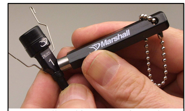
Turning Off: Hold magnet to base of transmitter until you hear 5 beeps.
